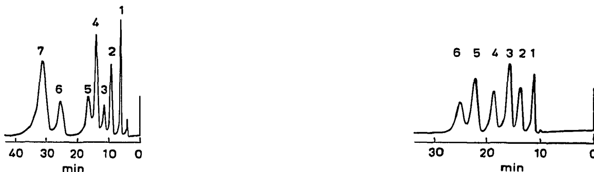
Fig. 2. Separation of tranquilizers by ion-pair chromatography. Support, 10- \mu m Merckosorb S1100; stationary phase, 0.1 M HClO 4 -0.9 M NaClO 4 loaded in situ ; eluent, chloroform-1-butanol (3:7); linear velocity, 0.5 mm/sec; sample, 1 \mu l containing 100-300 ng of each solute. Solutes: (1) nortriptyline; (2) trimipramine; (3) propiomazine; (4) pipamazine; (5) thiopropazate; (6) perphenazine; (7) opipramol.
