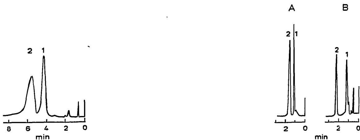
Fig. 4. Separation of trimipramine (1) and imipramine (2) by adsorption chromatography. Adsorbent, 20- \mu m Spherisorb AY; eluent, methylene chloride- n -pentane-acetic acid (79:20:1); linear velocity, 1.0 mm/sec; sample, 2 \mu l containing 0.3–3 \mu g of each solute.
